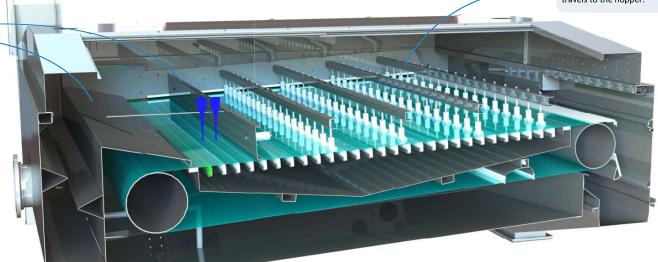
**Filtrate drains** to the bottom and out through the filtrate outlet.
